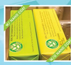
Color fading shown on the same packaging due to UV ray exposure
